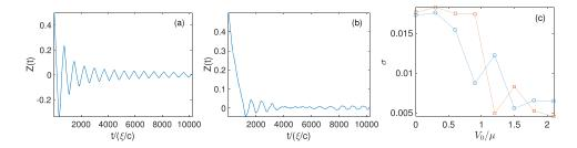
**Figure 7.** Panel (a) evolution of relative density Z(t) for parameters  $V_0 = 0.0$ ,  $\sigma = 1.2$  and  $Z_0 = 0.49$ . Panel (b) the same for  $V_0 = 1.5$ ,  $\sigma = 1.2$  and  $Z_0 = 0.49$ . Panel (c) the standard deviation of Z(t) after  $t_s = 4200\xi/c$  for a range of different barrier heights. The blue line with circles is for  $Z_0 = 0.49$  and the red with squares  $Z_0 = 0.88$ .
