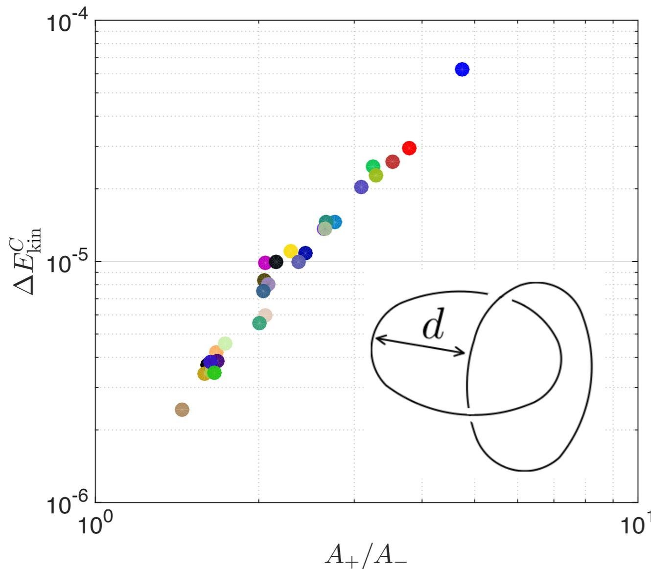
Growth of the compressible kinetic energy during the reconnection vs. the ratio  $A^+/A^-$  for the 49 different realisations
