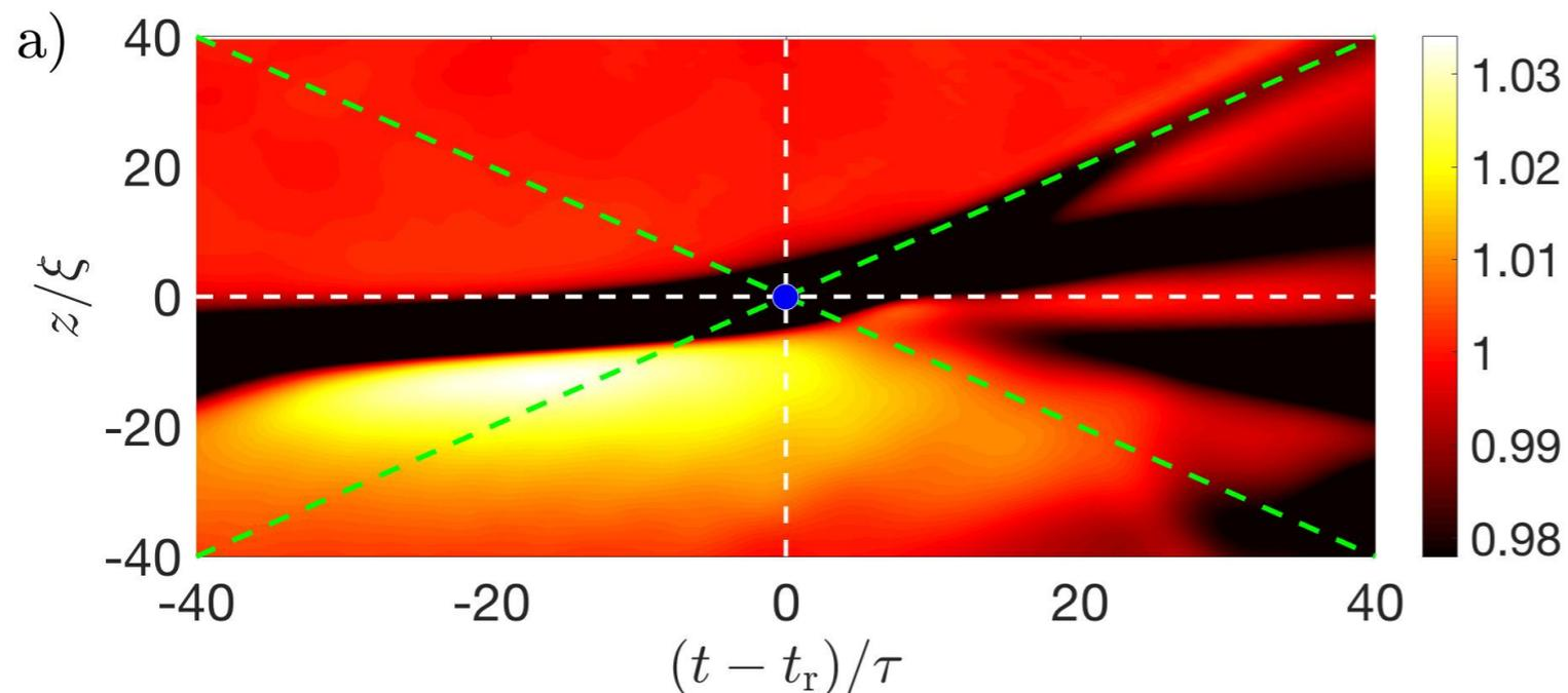
Example of sound pulse emission propagating orthogonally to the reconnection plane
