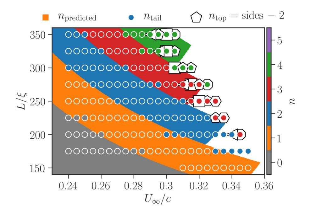
Number of vortices generated depending on the speed and length parameters. The curves indicate the phenomenological prediction. The white area indicate the stalling behaviour
