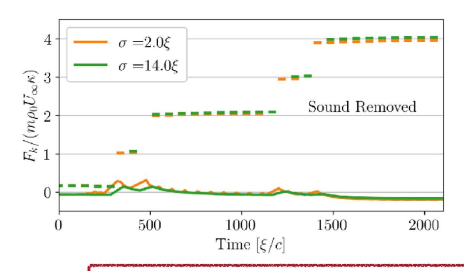
Rescaled lift (dashed) and drag (solid) versus time computed for different contours around the airfoil removing sound
