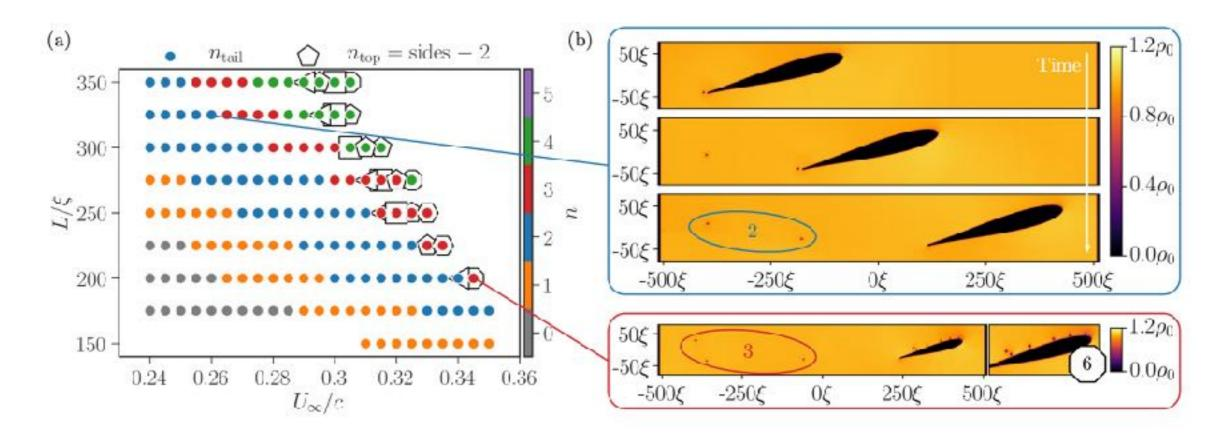
Left: number of vortices produced at the trailing edge. Vortices produced at the top are highlighted with a polygon. Right: two simulation examples, the latter with the detachment of the boundary layer causing a stall condition.
