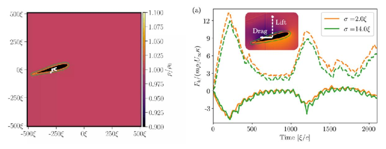
Left: video showing the sound emission during the vortex nucleation at the trailing edge. Right: rescaled lift (dashed) and drag (solid) versus time computed for different contours around the airfoil.
