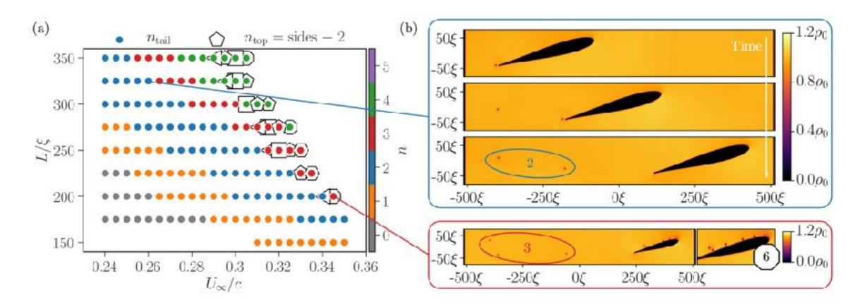
Left: number of vortices produced at the trailing edge. Vortices produced at the top are highlighted with a polygon. Right: two simulation examples, the latter with the detachment of the boundary layer causing a stall condition.
